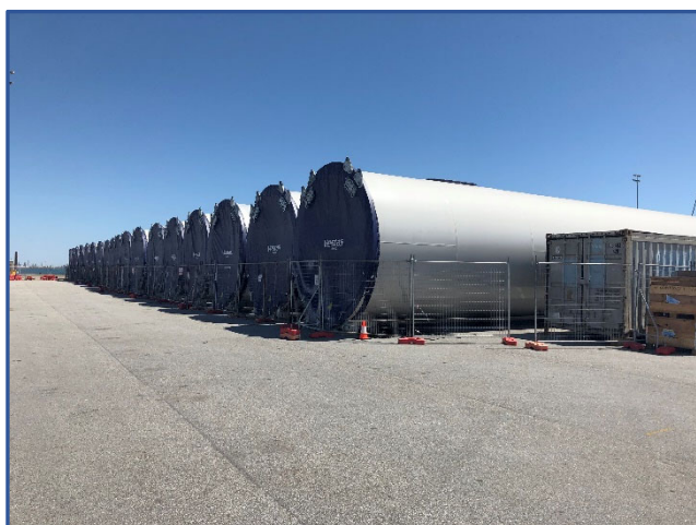
Tower sections stored at Henderson
